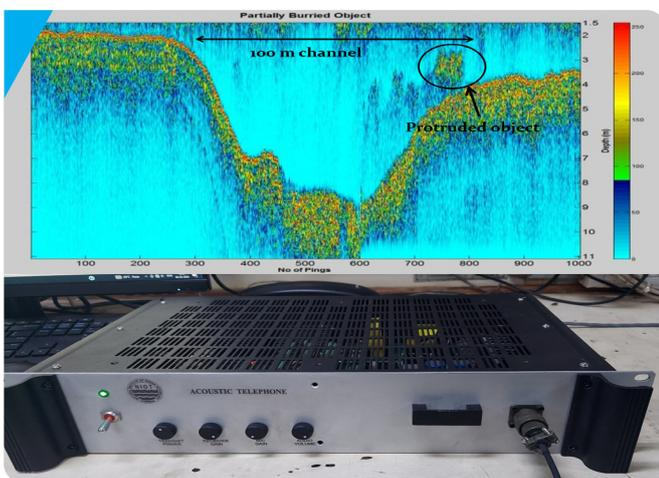
Indigenously designed and developed digital processing based prototype Acoustic Telephone for two-way voice communication demonstrated in offshore Bay of Bengal at approximately 500m depth and indigenous acoustic sub-bottom profiler for shallow water application was developed and demonstrated off Chennai coast.
