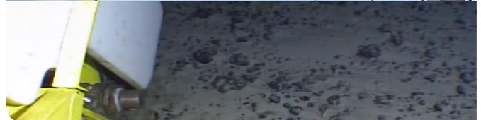
Demonstration and collection of polymetallic nodules in a first of its kind mining trials off Nicobar in West Sewell ridge using VARAHA-3 in 1200m water depths.
