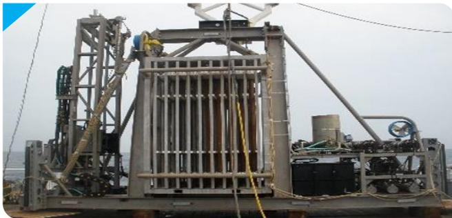
Deployment and drilling operation of Autonomous Coring System (ACS) at Krishna Godavari Basin site in 1060m depths and coring upto 60m below the seabed.
