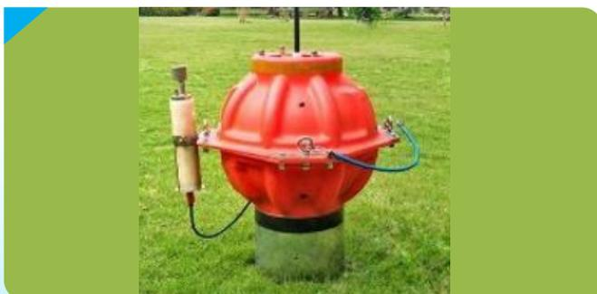
Indigenous design and development of Deep Sea Autonomous Underwater Profiling Drifter (DAUPD) float - successfully tested in 110m depth.
