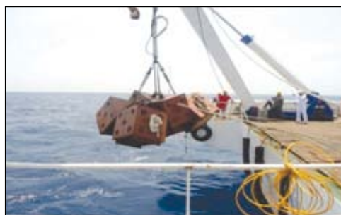
Winch testing with dummy load
