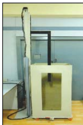
Tsunami Test Rig
