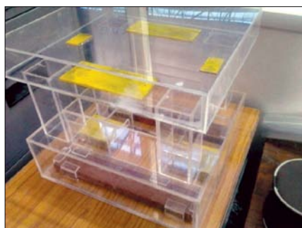
Physical model of Semi submersible with 4 column ring pontoon
