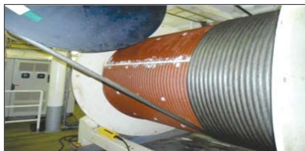
Umbilical cable winding in modified LEBUS of winch in initial stage
