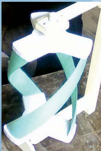
Ø157 mm Gorlov turbine model made from Rapid prototype machine (3D printing)
