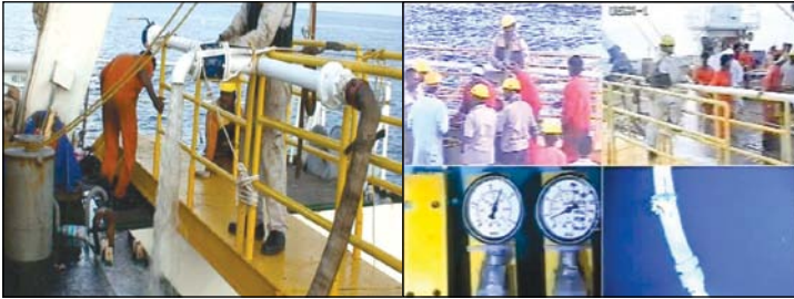
Water being pumped from 616 m depth Observation of solids pump performance
