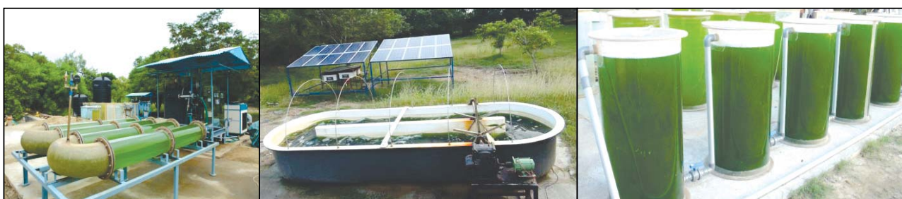
Tubular PBR with control system
