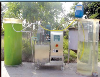
Tubular Photobioreactor with process controller
