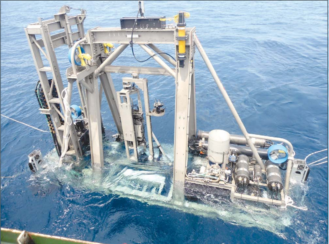
Autonomous coring system being launched from the vessel
