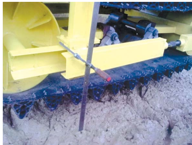
Pull out tests of undercarriage
