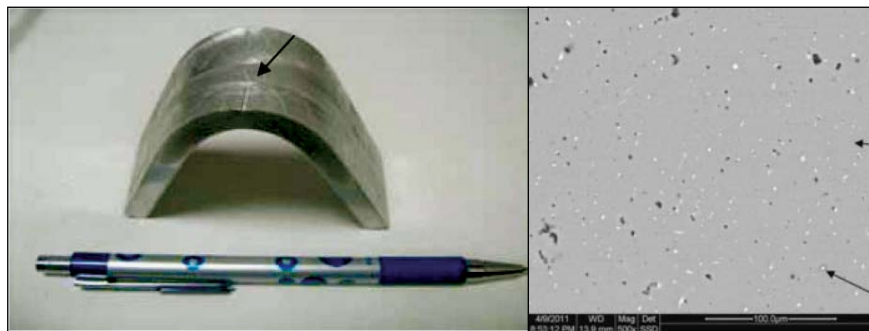
Bent specimen (5083 multi - pass weld)
