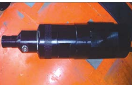
Anodized cable collectors re-installed in TMS pressure case
