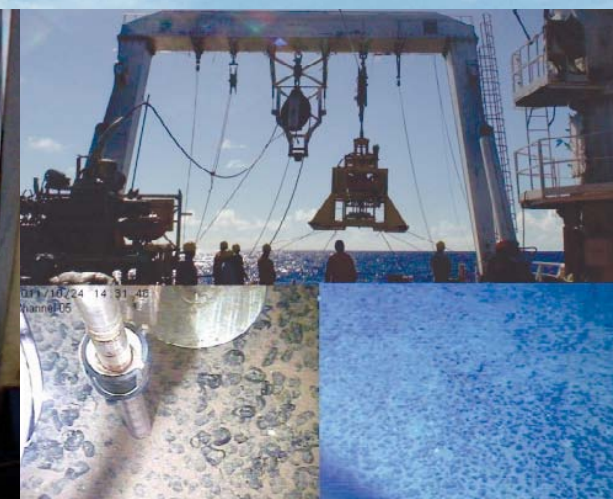
Launching of ROSIS from Sagar Nidhi and view of nodules from 5462 m depth
