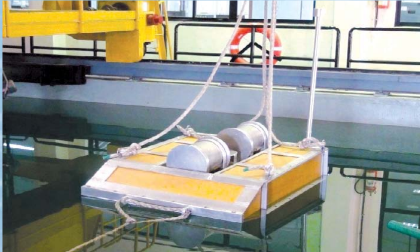
Tow body during Buoyancy Test
