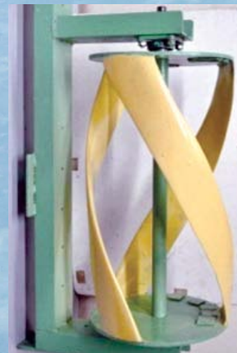
Ø300 mm helical turbine made of steel reinforced blades
